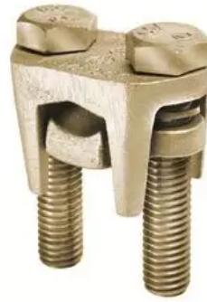
Compact, two-piece, high strength, high copper alloy BURNDY OKLIP recommended for heavy duty connections. Neoprene rings hold DURIUM bolts in place during installation. Installed with ordinary wrench. Recommended tightening torque: 250 in-lb.
